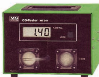
MSWT201 Messer CO Tester Measurement Range : 0 - 10.0 % Reading Range : 19.9 % Resolution : 0.1 % Warm up Time : < 60 seconds Power Supply Car Battery : 10 - 16 Volts Dimensions : 145 x 200 x 200 mm Weight : 2.8 Kg
