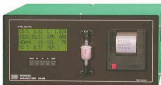
MSG540 Messer Infrared 4 Gas Analyser Siemens Gas Bench Measures : CO, CO 2 , HC, O 2 Lamda Factor Calculation Warm up Time : 9 minutes Automatic Self Calibration
