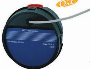
BG102101 1/2" Pulse Meter 70 Bar 0 - 35 l/m 100 ppl Reed Switch Output
