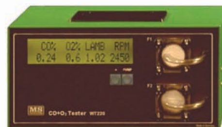
MSWT220 Messer 2 Gas Tester RPM, CO & O 2 Measurement Lamda Factor Calculation
