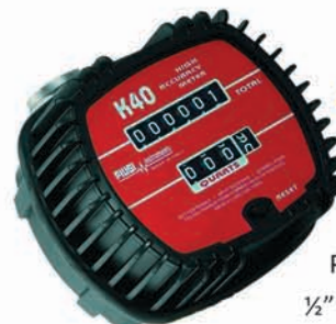
BG102900 3/4" Digital Oil Meter 100 Bar 0 - 60 l/m Accuracy \pm 0.5\% Calibration Facility
