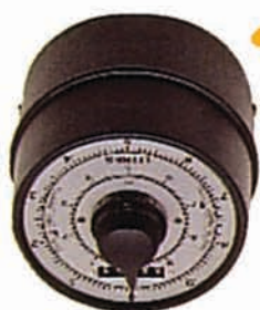
BG103042 1/2" Oil Meter 70 Bar 0 - 15 l/m Accuracy \pm 0.5\%
